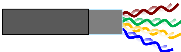
Slika 50. F/UTP kabel (Eng. Foiled with Unshielded Twisted Pair)
