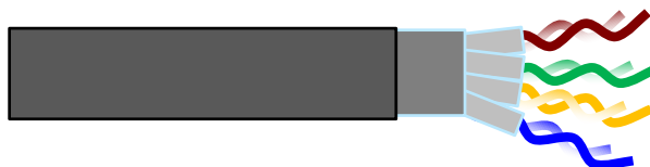
Slika 54. F/FTP kabel (eng. Shielded and Foiled with Unshielded Twisted Pairs )
